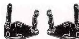
HOOD HINGE BRACKETS - 1938/'40 & 1940/'41 DELIVERY Available in powder coated glass black or polished stainless steel.
