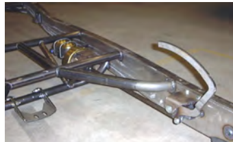
#70013 Trans Mount for 700R4 (rubber insulator sold separately - see below)
