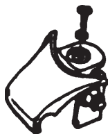
FRONT FENDER TIE BRACKETS - Die Cast!! This clamps the front fenders together under the front grille. All hardware included.
